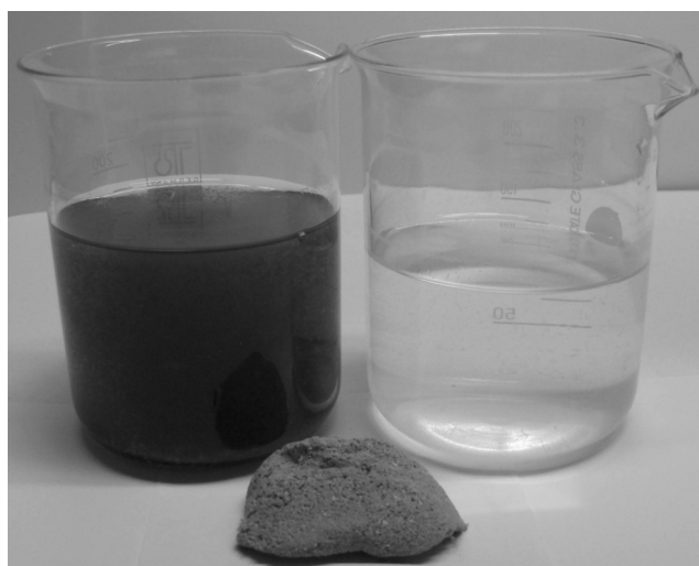
Fig. 8. Left: Starting textile industry wastewater, Centre: Odorless and cohesive zeo-sludge and Right: Clear water after the HENAZE treatment.
