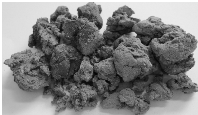
Fig. 5. Odorless and cohesive zeo-sewage sludge (proportions 50:50, after 36 hours at RT).
