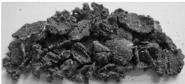
Fig. 4. Odorless and cohesive zeo-sewage sludge (proportions 80:20, after 18 hours at 105 °C).
